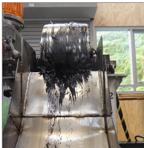
Magnetite concentrate on Low Intensity Magnets (LIMS)
