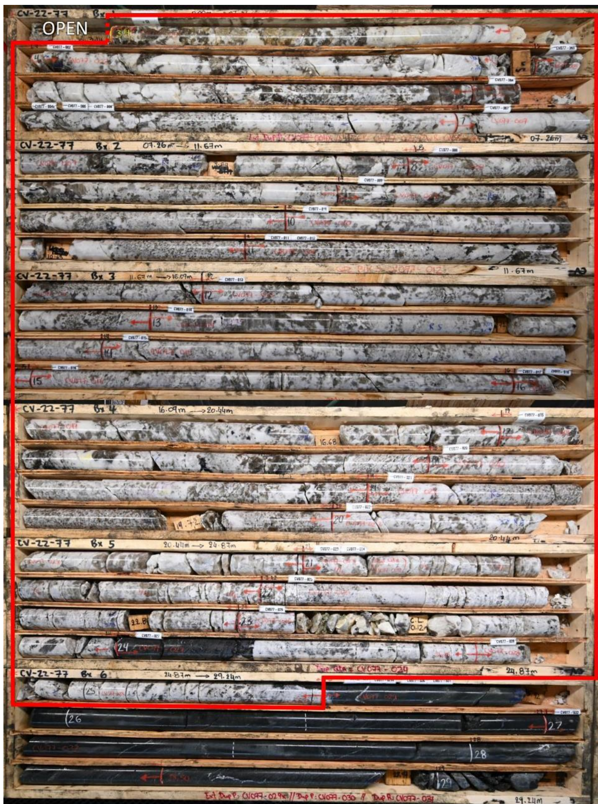
Figure 4: Spodumene drill-core intersection in drill hole CV22-077 (22.4 m at 1.28% \text{Li}_2\text{O} ), which collared in spodumene pegmatite.
