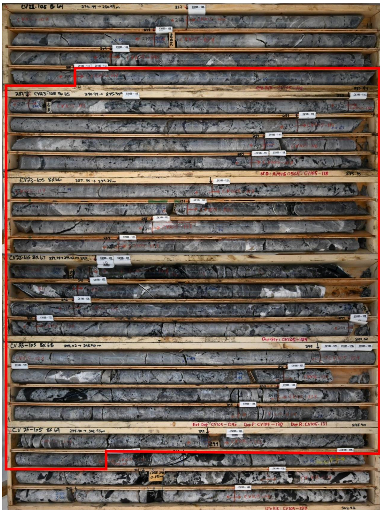
Figure 2: High-grade lithium pegmatite intersection in drill hole CV23-105 – 19.8 m at 5.28% Li 2 O (red box)
