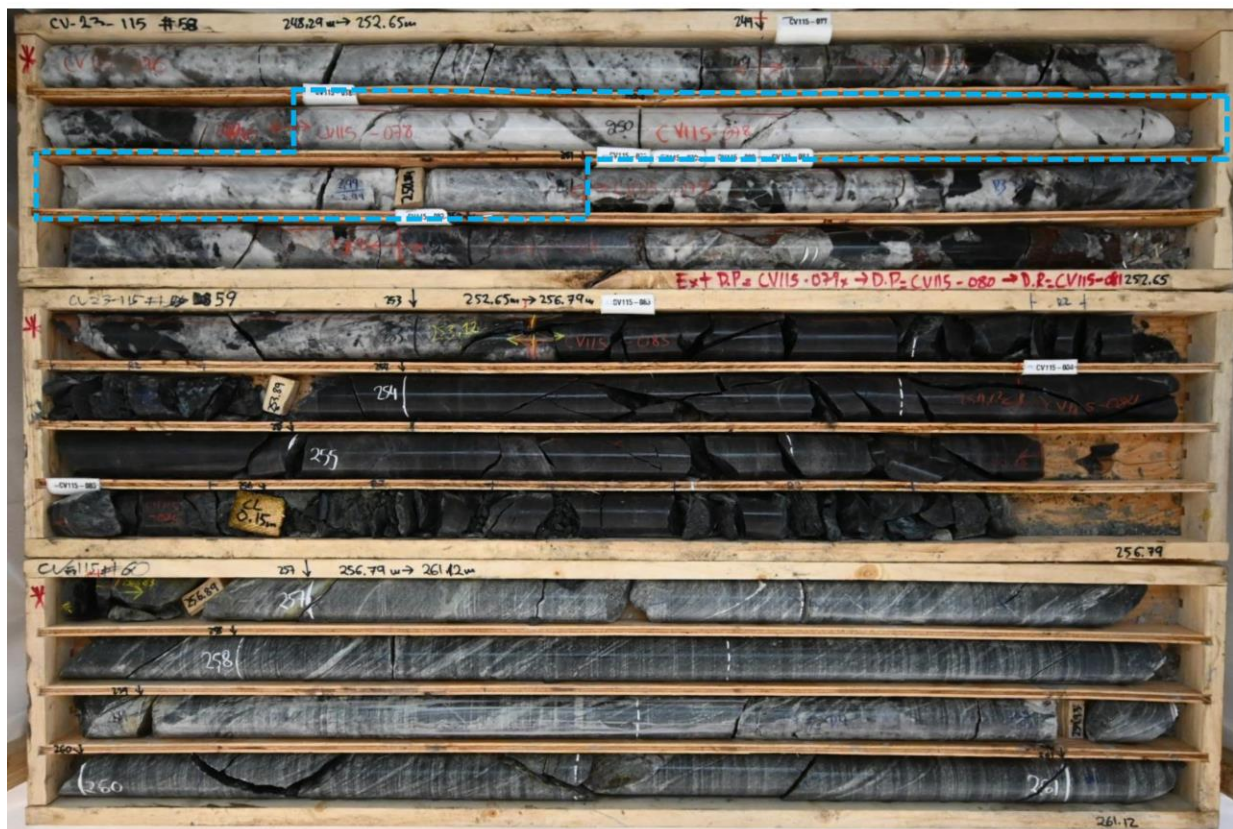
Figure 3: Spodumene in pegmatite from drill hole CV23-105 (top), and high-grade lithium pegmatite intersection in drill hole CV23-115 (bottom) – 1.3 m at 6.53% \text{Li}_2\text{O} (blue box)
