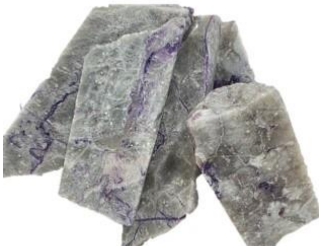
Figure 4: High grade pollucite drill core from the Vega Zone, assaying ~30% \text{Cs}_2\text{O} . Sample is a targeted selection of pollucite from a drill core composite sample, which was used as a training sample for the XRT ore sorter software. See Table 1, Figure 5, and news release dated April 9, 2025 , for drill hole composite sample intervals, location, and assay data.
