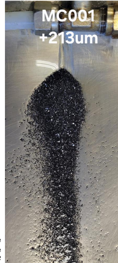
Concentrate from Mozley table testwork from CV5 drill core composite MC001 2
