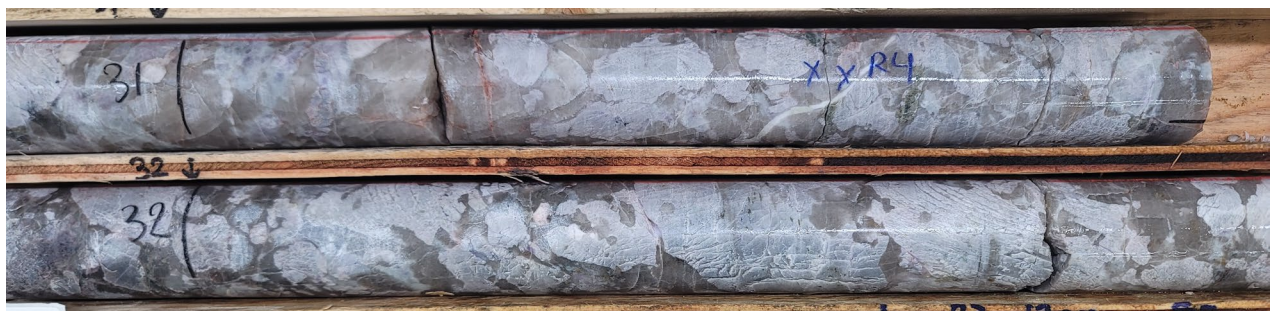
Figure 5: Large spodumene crystals in drill hole CV25-875 at ~32 m depth (core length) at the CV12 Pegmatite. Core graded 2.9 m at 2.70% Li 2 O over sample interval (30.1 m to 33.0 m).
