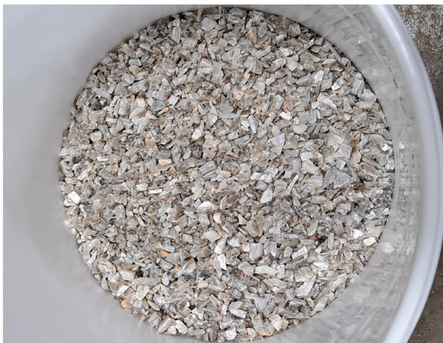
Figure 7: DMS spodumene concentrate (after magnetic separation) assaying 6.32% \text{Li}_2\text{O} and 0.45% \text{Fe}_2\text{O}_3 .
