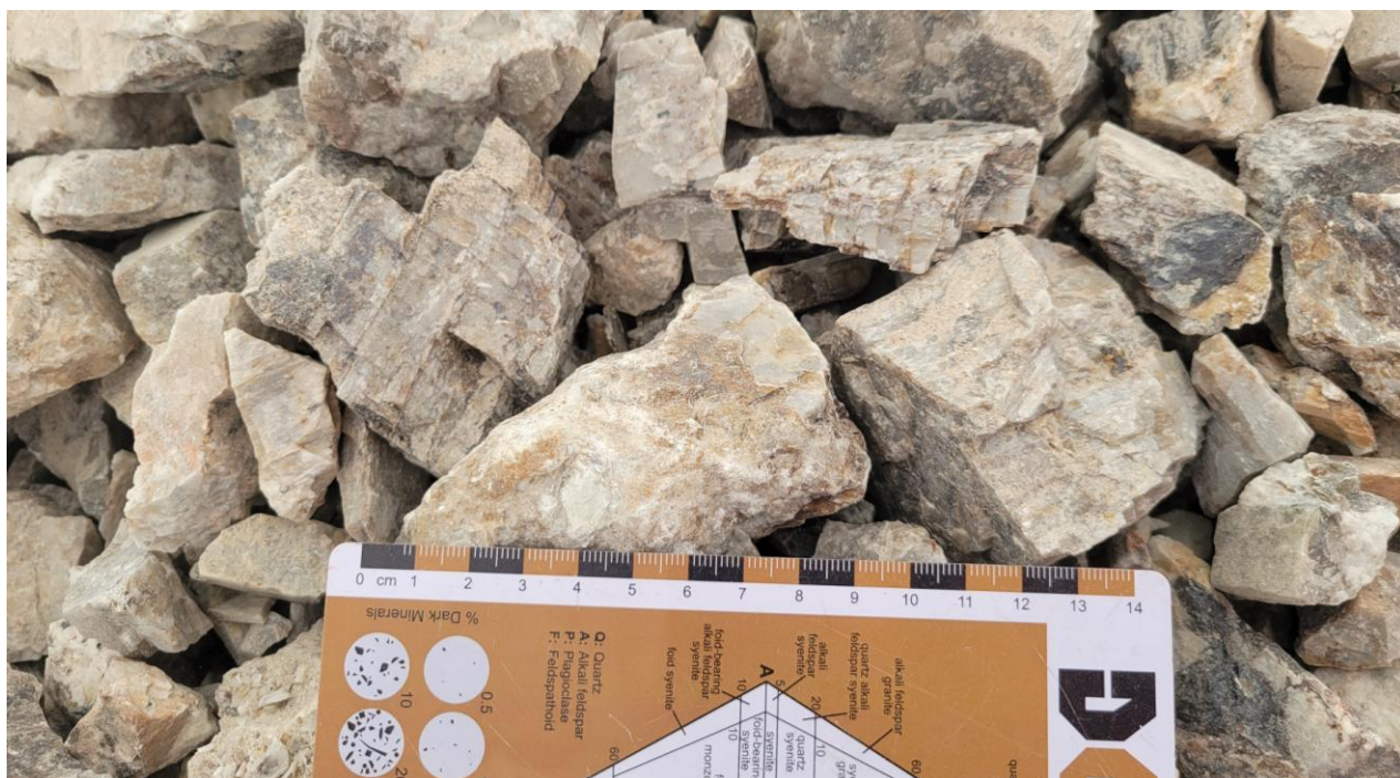
Figure 5: Crushed spodumene pegmatite ready for shipment to the SGS (Lakefield) facility in Ontario for DMS processing with a head-grade assaying 3.61% \text{Li}_2\text{O}
