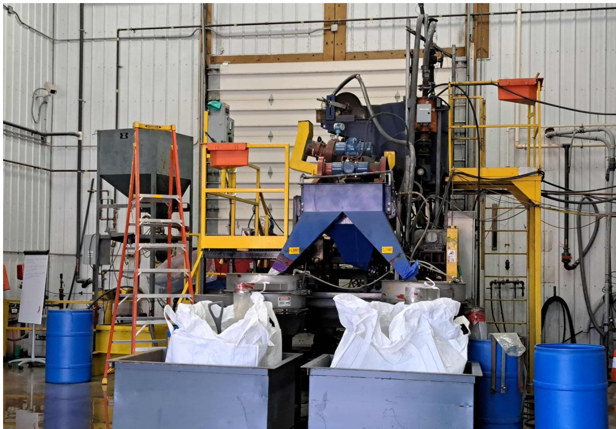
Figure 6: Dense Media Separation (“DMS”) pilot operation at SGS (Lakefield) facility in ON, Canada.
