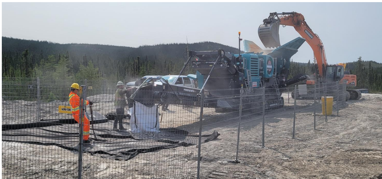
Figure 4: Crushing of spodumene pegmatite boulders into bulk bags.
