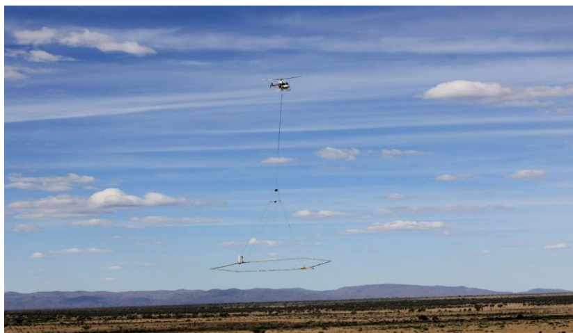
Helicopter SkyTEM Survey 2011 - Musgrave Project
