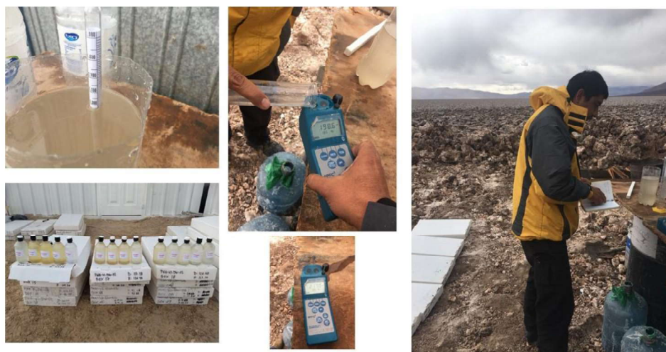
Photo 1 - Field parameter recording of samples for conductivity, density, Ph and temperature
