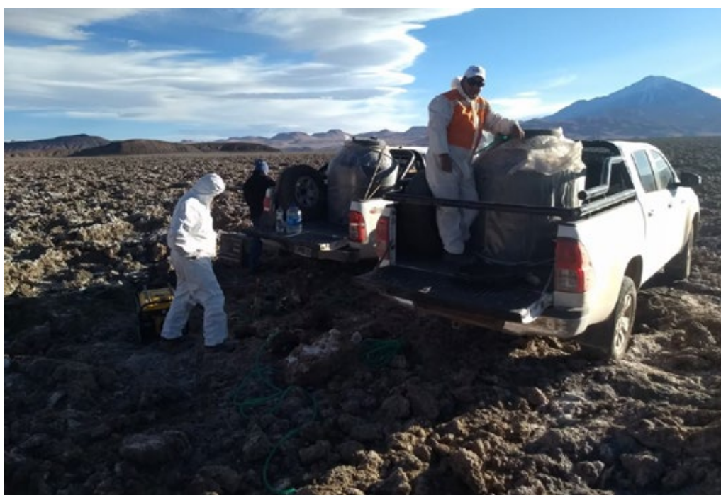
Photo 1 – Salar de Incahuasi - Brine Collection by pumping from trenches created Aug-Sep 2019
