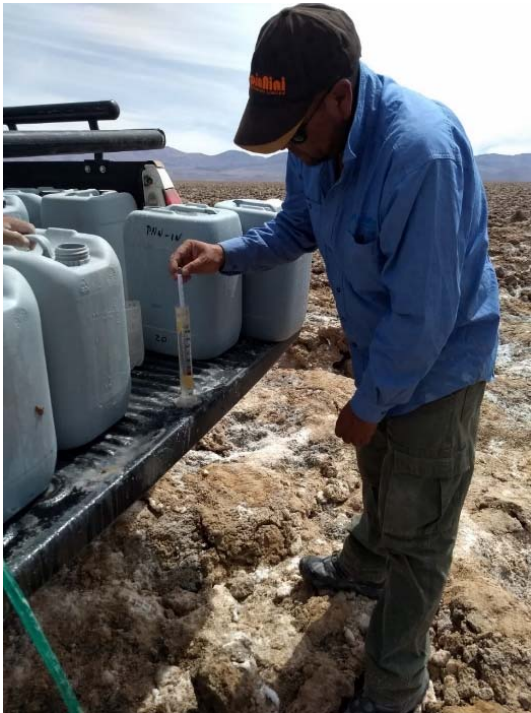
Photos 3 and 4 - Relative density of brine measured before labelled plastic brine containers were sealed for transport
