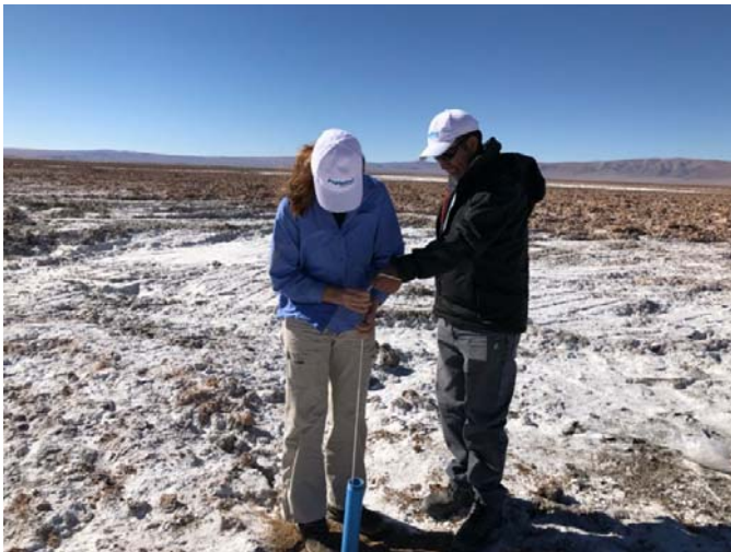
Photo 2 - Salar de Rincon - Brine was pumped from monitoring wells converted from resource drilling program Dec 2017
