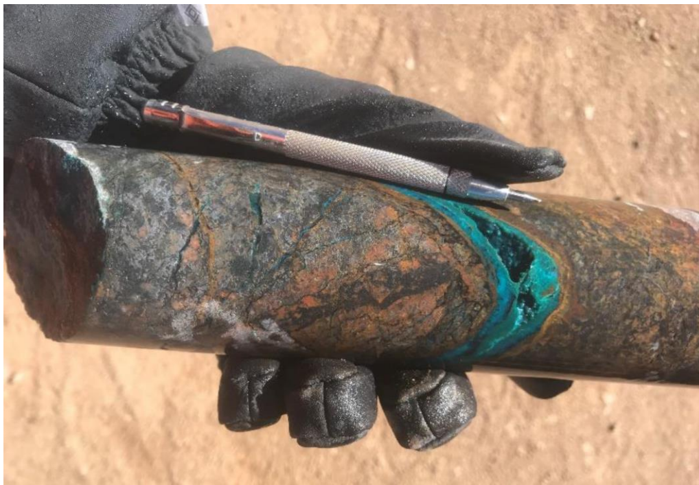
Figure 6: Drill core from hole PNSI22-001 at 89m showing quartz-malachite-azurite-chrysocolla veins
