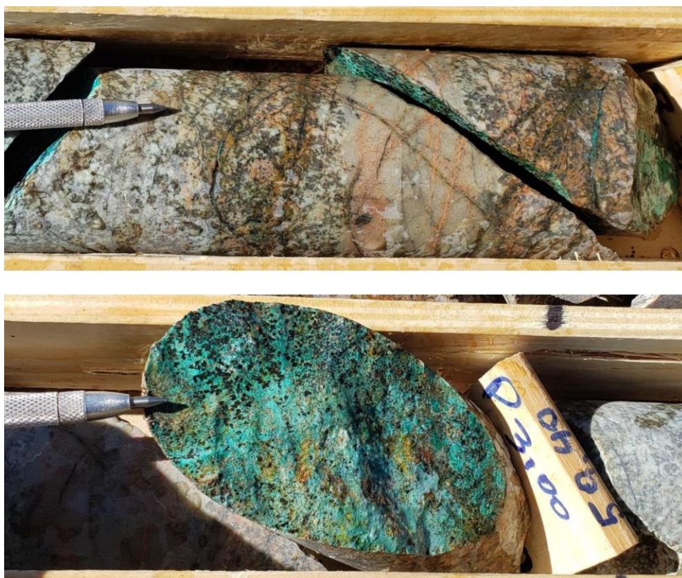
Figure 7: Drill core from hole PNSI22-002 at 59.4m showing quartz-biotite-magnetite veins with Cu-Fe oxides
