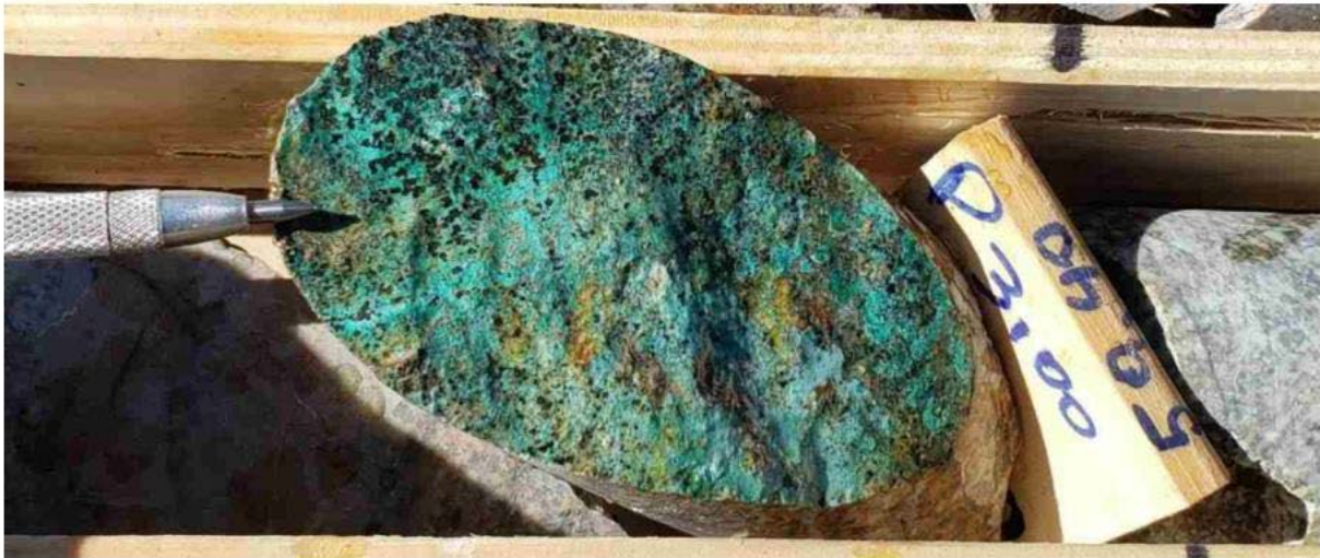
Drill core from hole PNSI22-002 at 59.4m showing quartz-biotite-magnetite veins with Cu-Fe oxides
