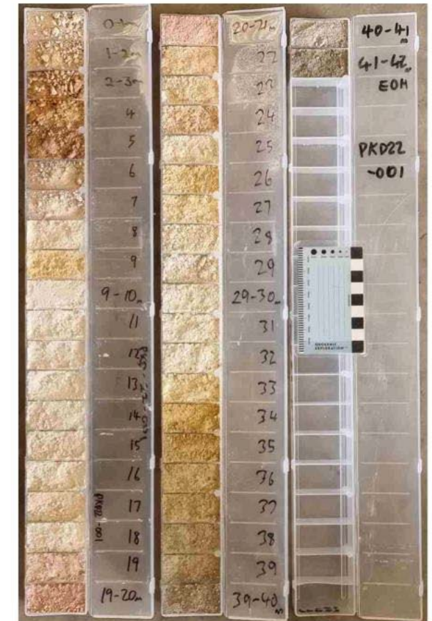
Chip samples from drill holes PKD22-008 (left) and PKD22-001 (right), Kapinnie (EL 6689) at Eyre Peninsula Kaolin-Halloysite Project
