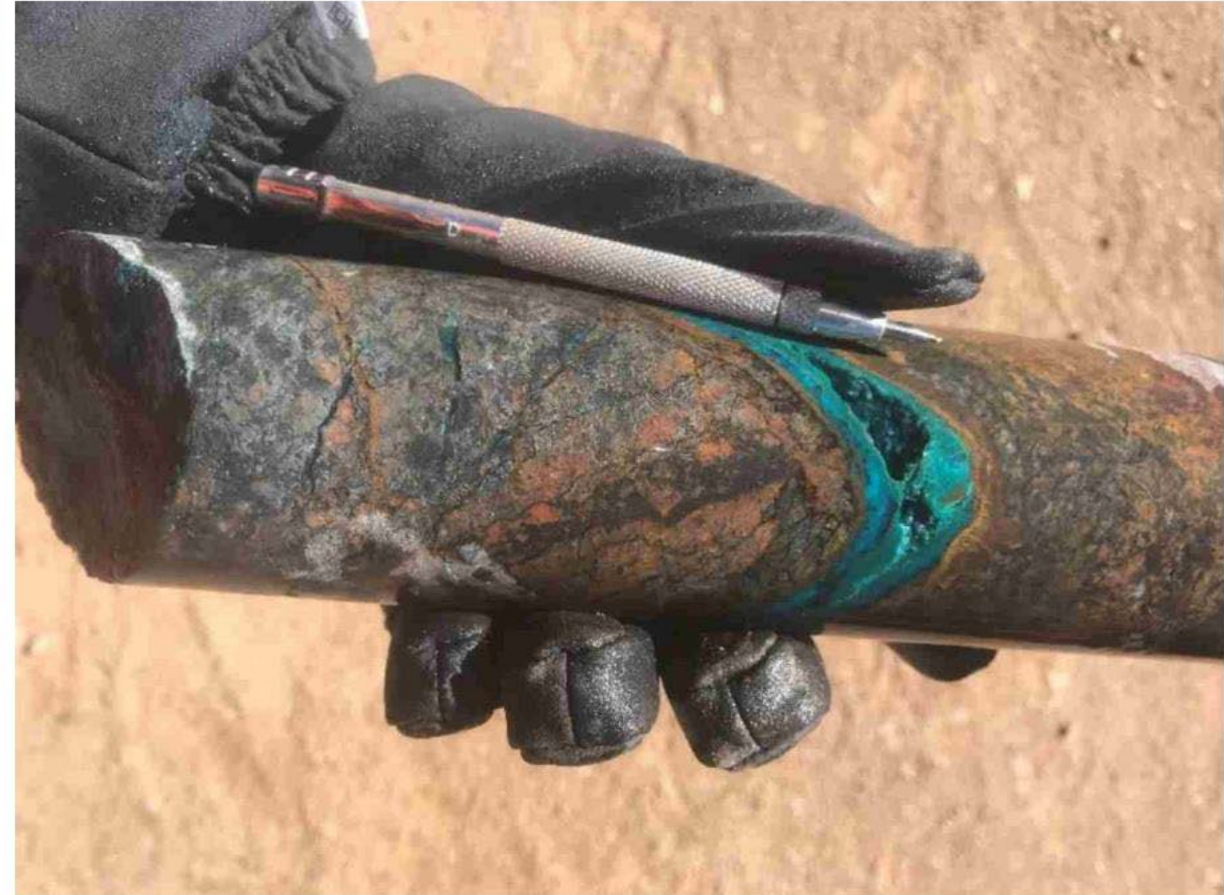
Drill core from hole PNSI22-001 at 89m showing quartz-malachite-azurite-chrysocolla veins
