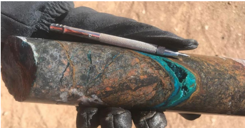
Figure 8: Drill core from hole PNSI22-001 at 89m showing quartz-malachite-azurite-chrysocolla veins
