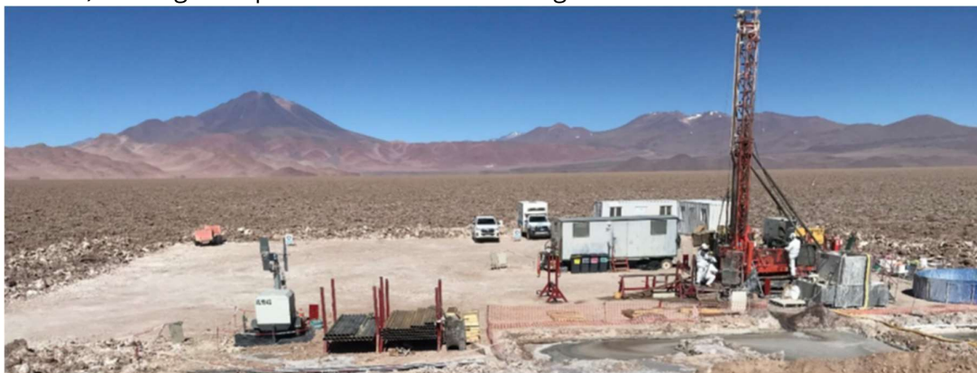
Figure 1: Resource drilling platform for drillhole PM22-IN-01 at the Incahuasi salar, Salta Lithium Project
