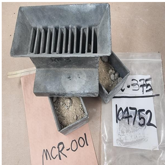
Figure 1: Drill sample splitting, Musgrave Nickel-Copper-Cobalt Project, Musgrave province, South Australia
