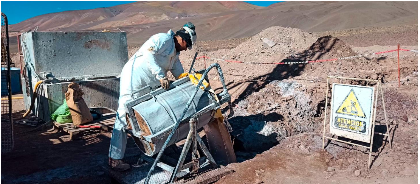
Figure 5: Brines packer testing at drillhole PM23-IN-04 at Incahuasi salar, Salta Lithium Project.
