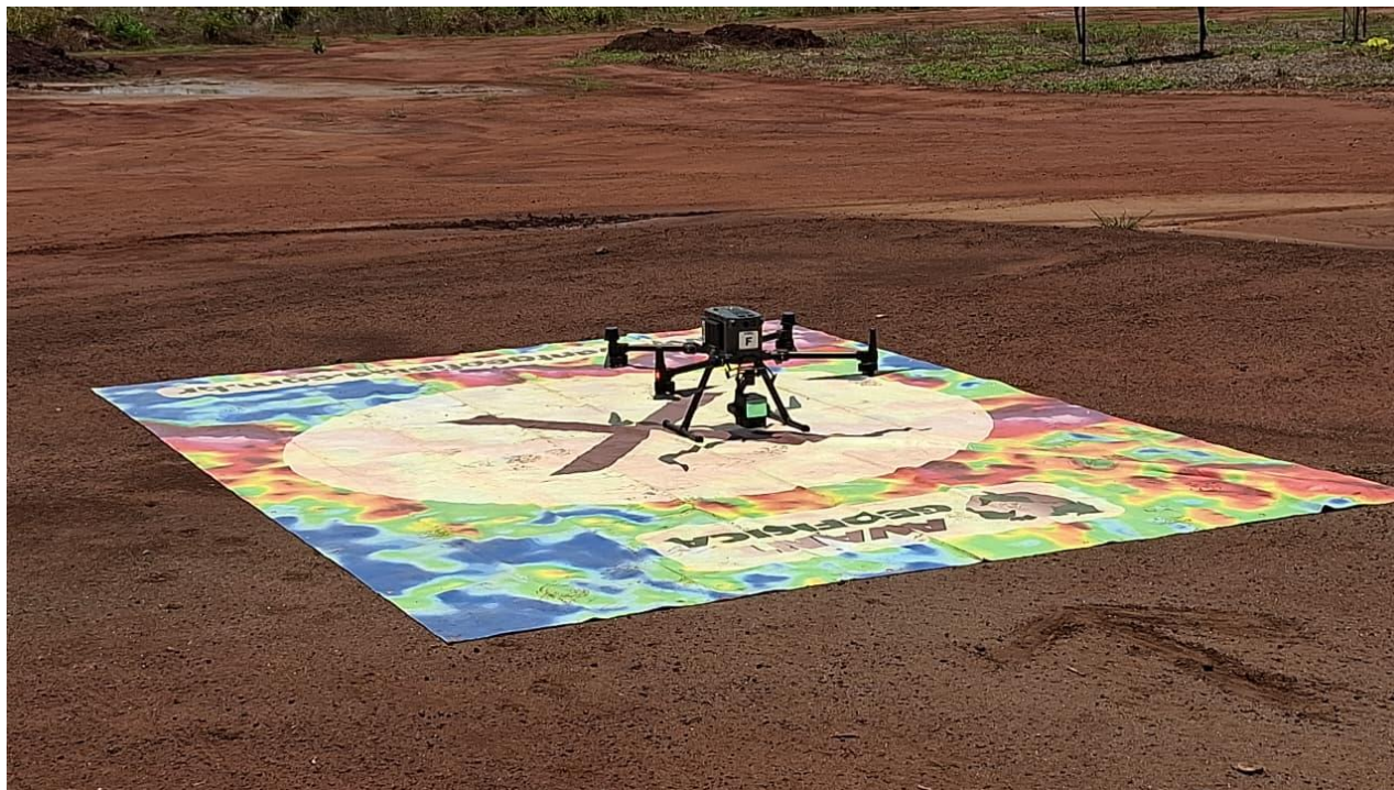
Figure 3: LiDAR sensor mounted below drone while on landing pad at Santa Anna
