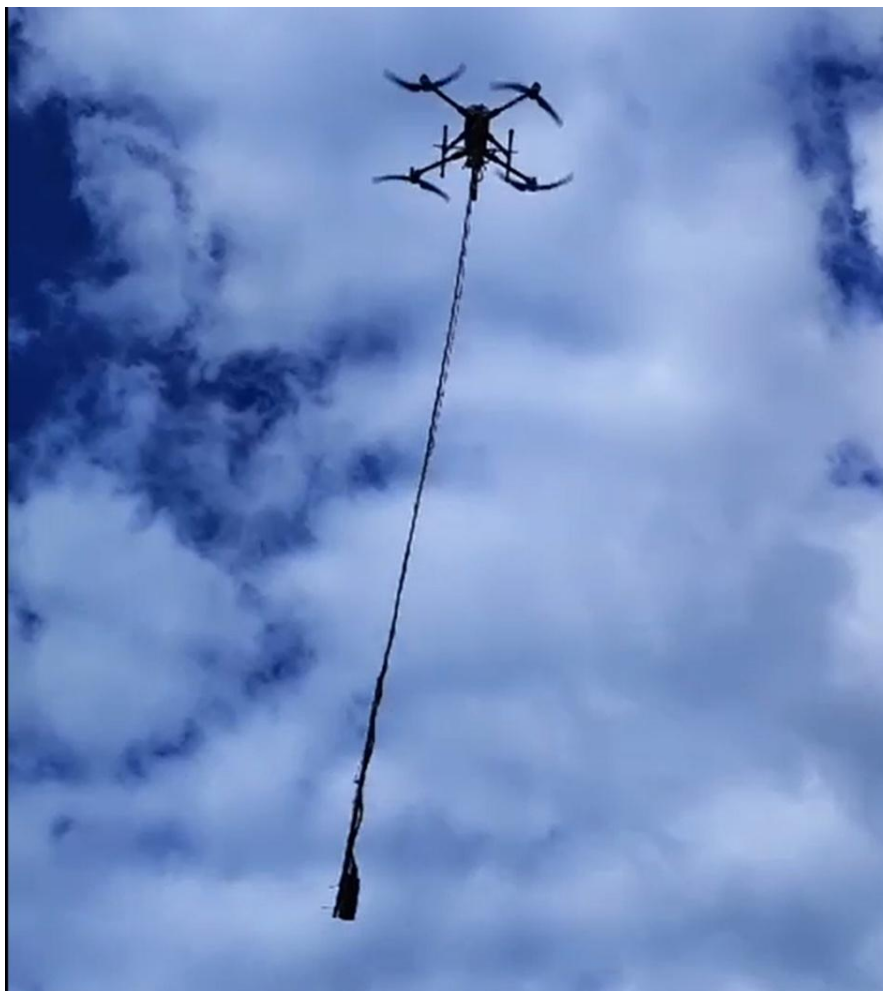
Figure 2: Magnetometer sensor below the drone at Santa Anna
