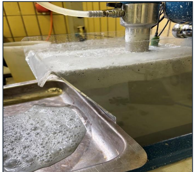
Figure 5: Rougher flotation (medium- and slow-floating PGM fraction)
