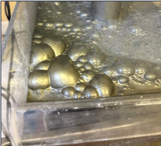
Figure 4: Flash flotation (fast-floating PGM fraction)
