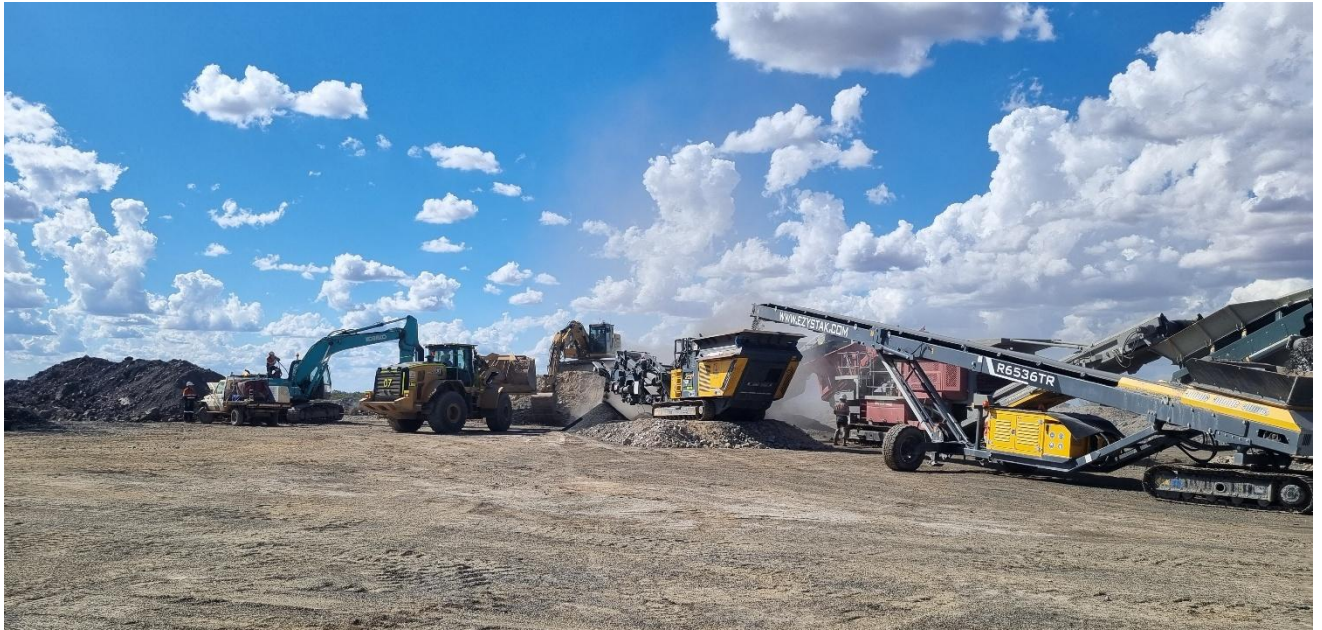
Figure 2. Crushing of UNL ore on ROM pad for direct shipment.
