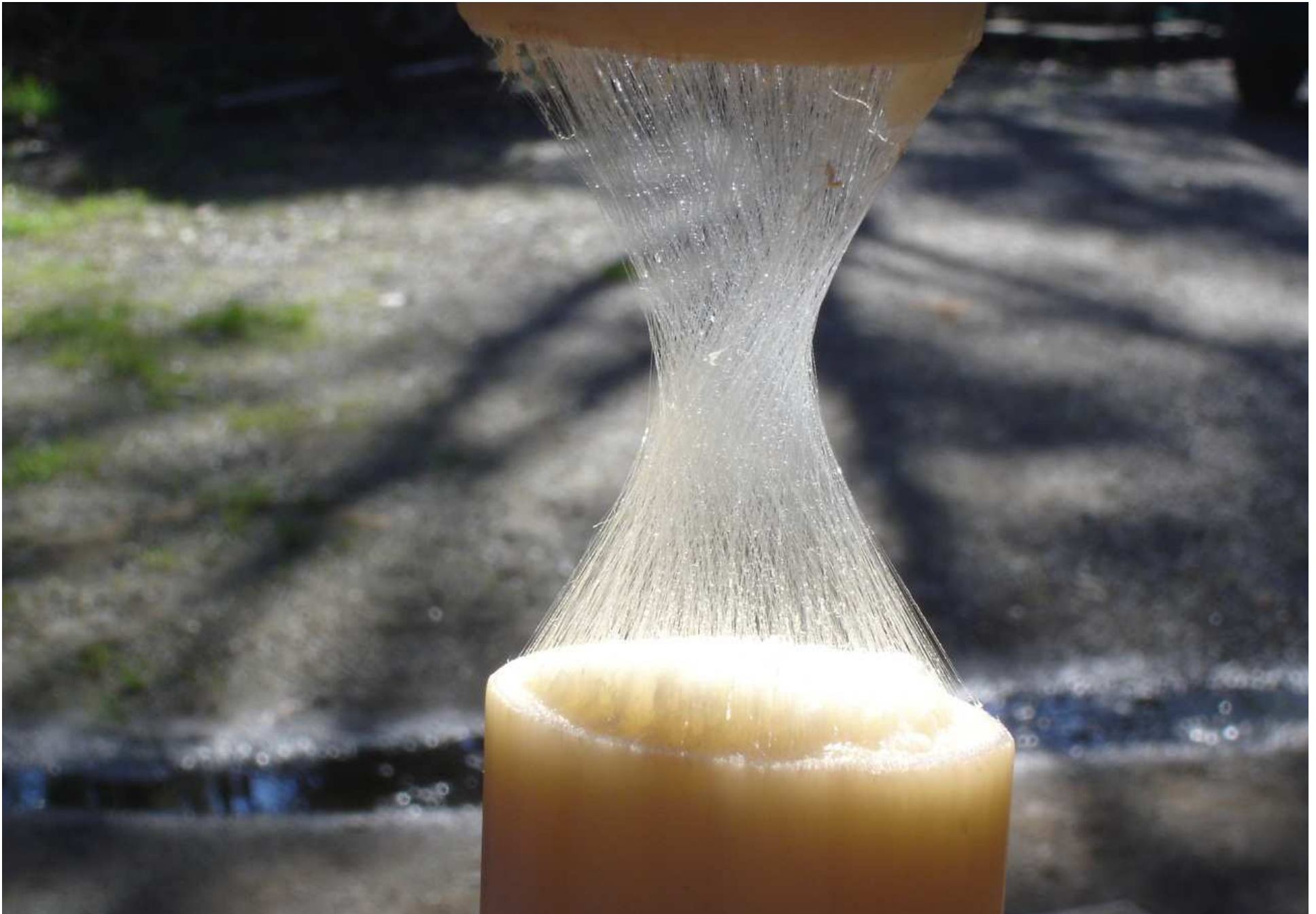
BANANA TREE TRUNK CORE FIBRE (LONG, STRONG & WHITE)
