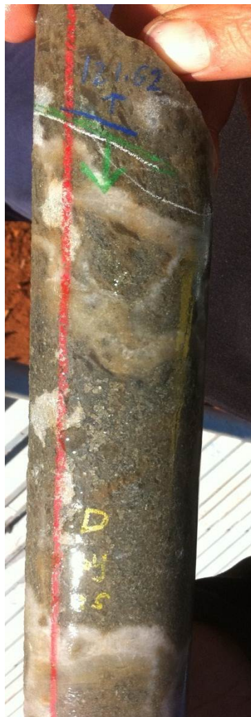
Intense sulphide development with high As / pyrite / alteration. Typical grade 1 to 10g/t Au.
