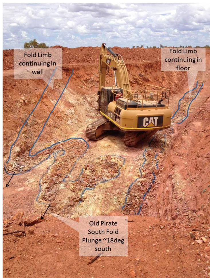
Figure 2. Old Pirate South fold nose exposed in pit floor and walls. Photo taken view NNW with the fold plunging south into the floor at 18 to 20 degrees.
