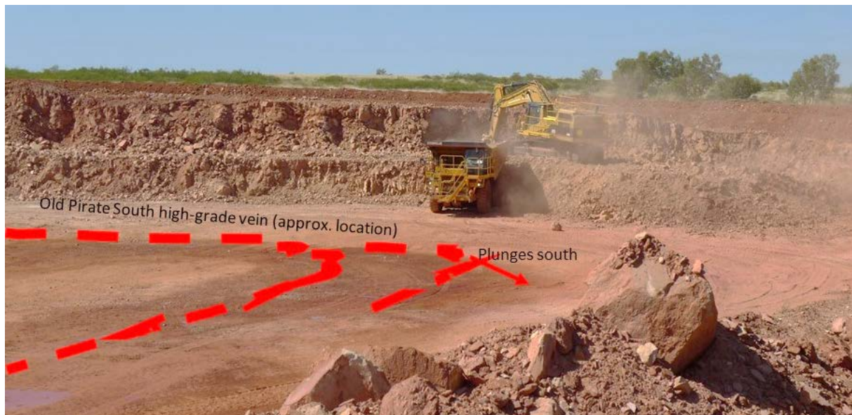
Figure 4. Old Pirate South Pit view east. Red lines annotate approximate location of high-grade veins
