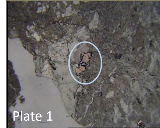
140001.04. Free gold interstitial to and overgrowing pyrite/arseniferous pyrite after granoblastic quartz-wallrock margin. 6mm. ppl/rl.
