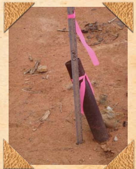
Diamond drill collar B10 at Mary Springs Mine
