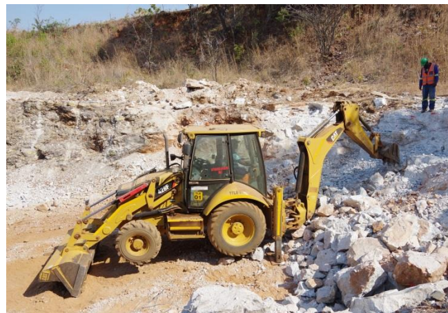
Blasted Main Pegmatite ready for stockpiling
