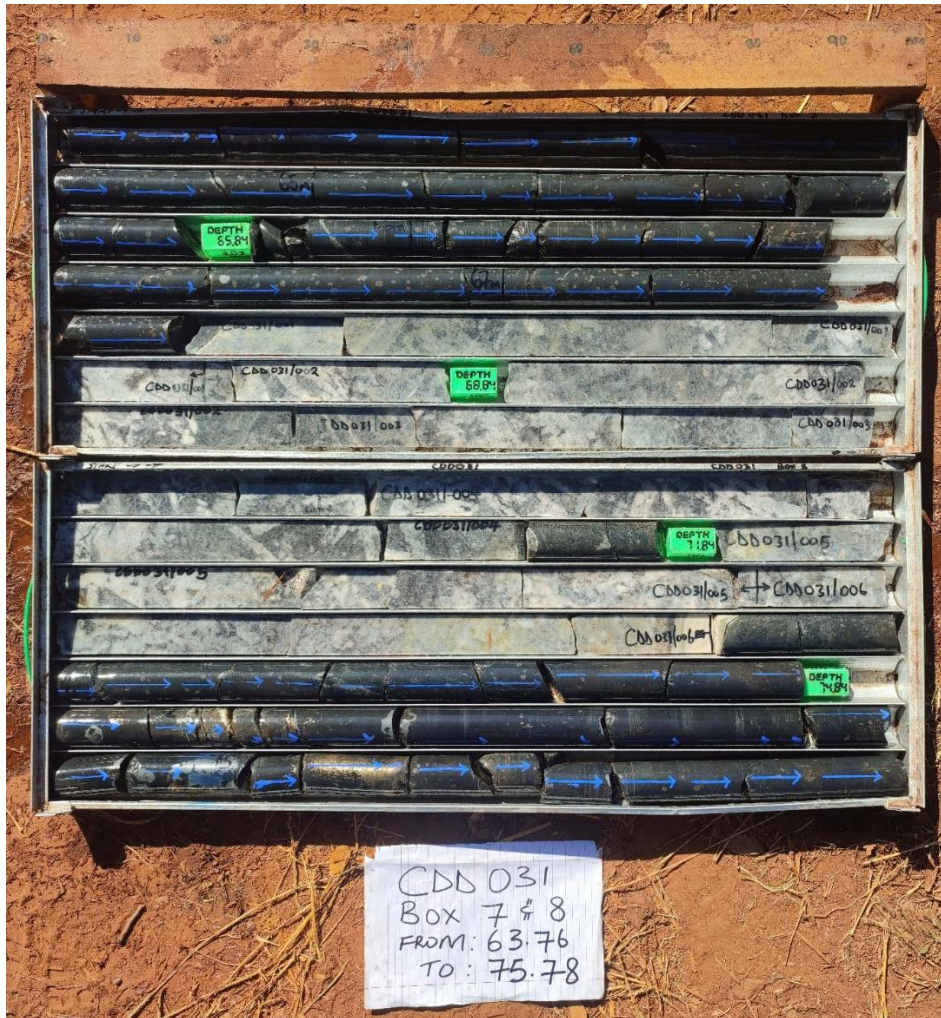
Figure 3: Wide zone of high grade lithium mineralisation in CDD031 (Pegmatite E)
