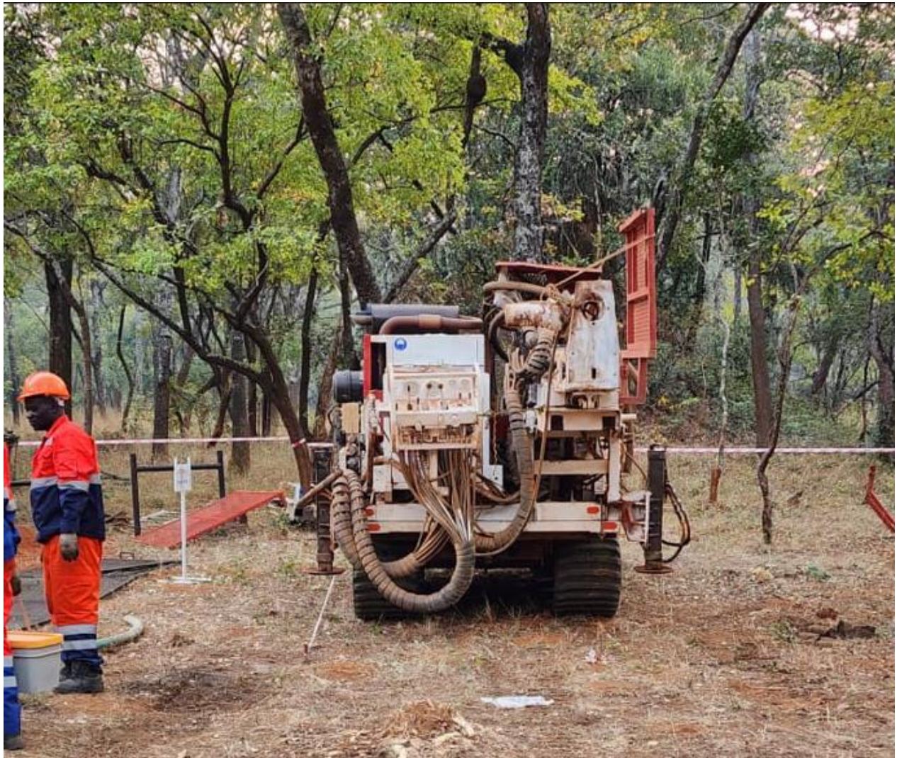
Figure 1: Diamond drilling rig on site at the Mumbezhi Copper Project
