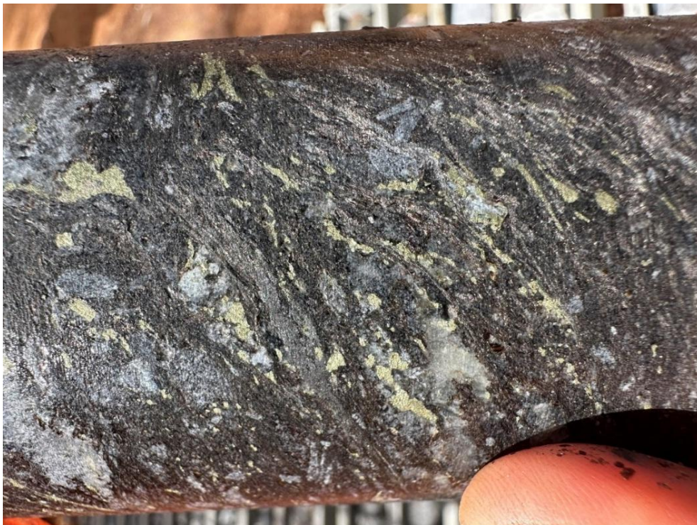
Figure 4: Chalcopyrite mineralisation intersected in a biotite-quartz-garnet-kyanite ore schist in NCRD009
