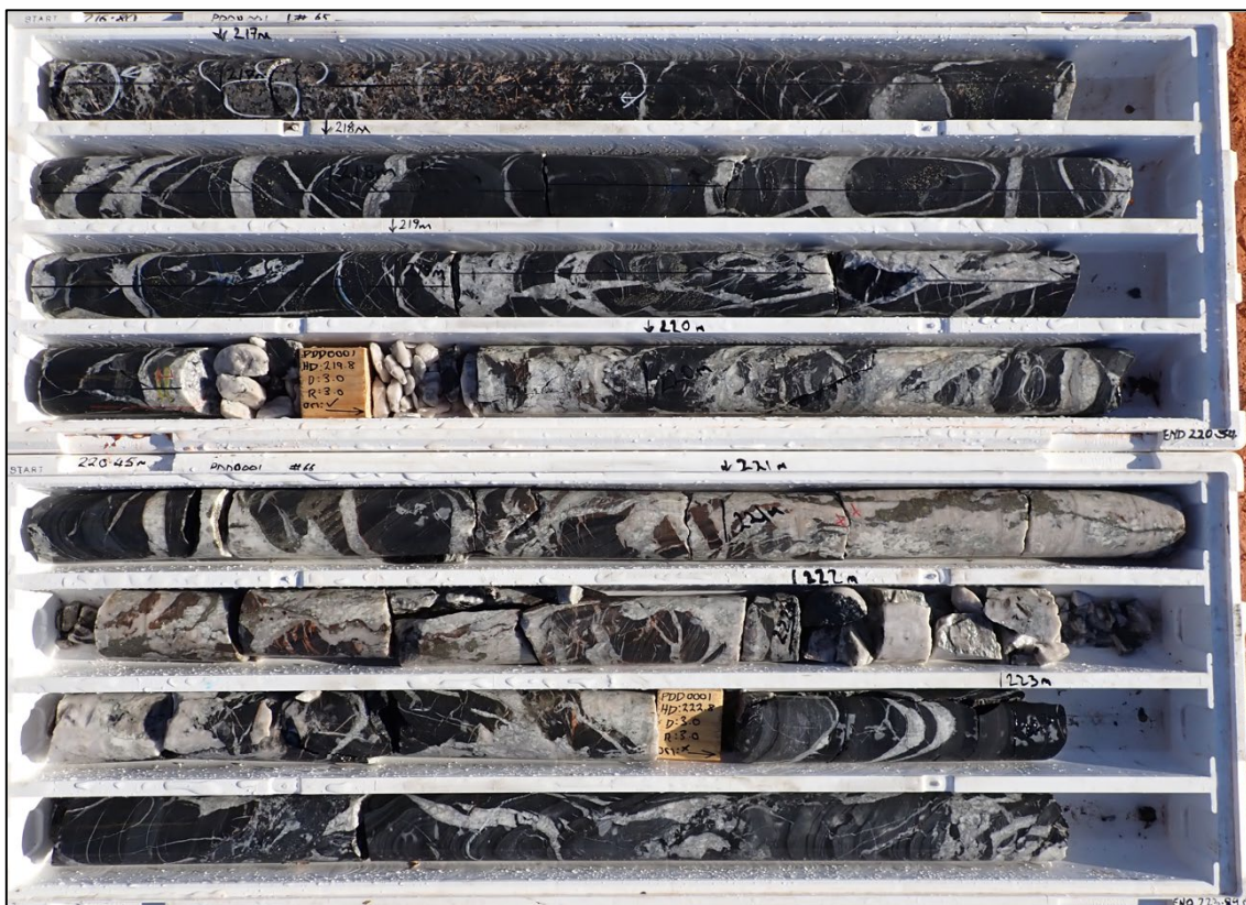
Figure 2: Core from PDD0001 showing quartz-carbonate veining and pyrite associated with the Grace/Bemm fault zone from 216.8m to 223.89m.
