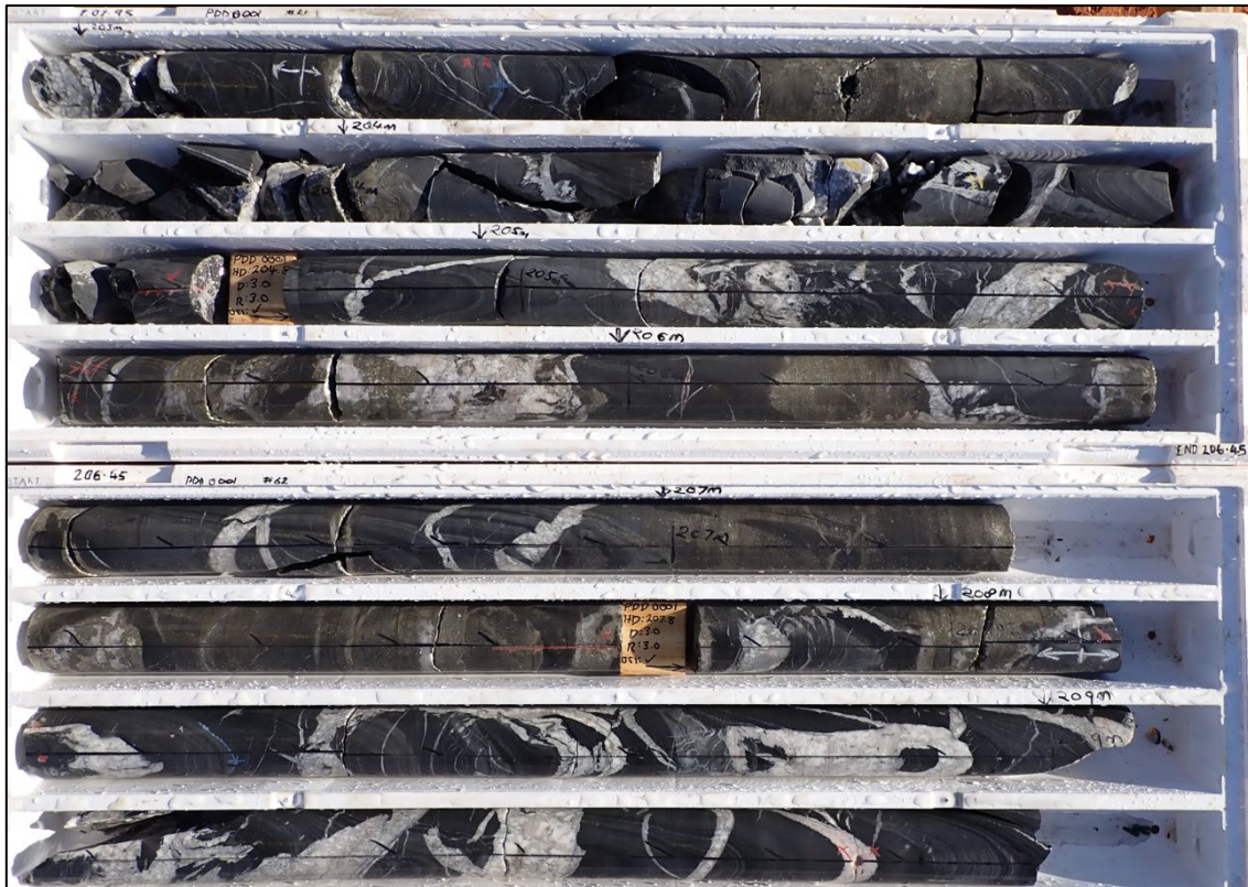
Figure 1: Core from PDD0001 showing quartz-carbonate veining and pyrite associated with the Grace/Bemm fault zone from 202.95m to 209.85m.
