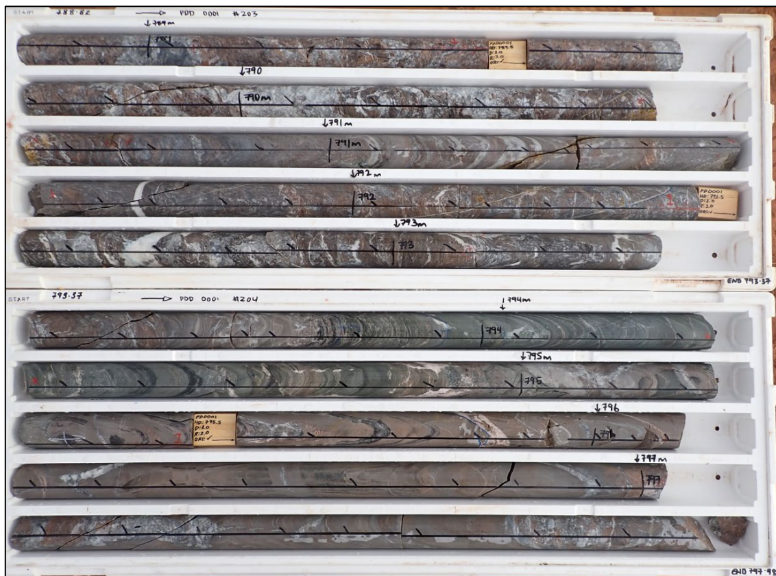
Figure 4: Core from PDD0001 showing intensely brecciated and altered core from 788.82m to 797.98m.
