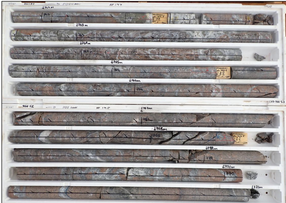
Figure 3: Core from PDD0001 showing minor quartz-carbonate-pyrite veining and a brecciated contact between altered sediments and a granitic unit. from 761.88m to 771m.
