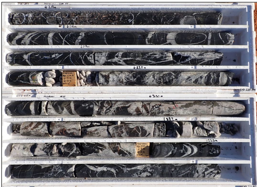
Figure 2: Core from PDD0001 showing quartz-carbonate veining and pyrite associated with the Grace/Bemm fault zone from 202.95m to 209.85m.
