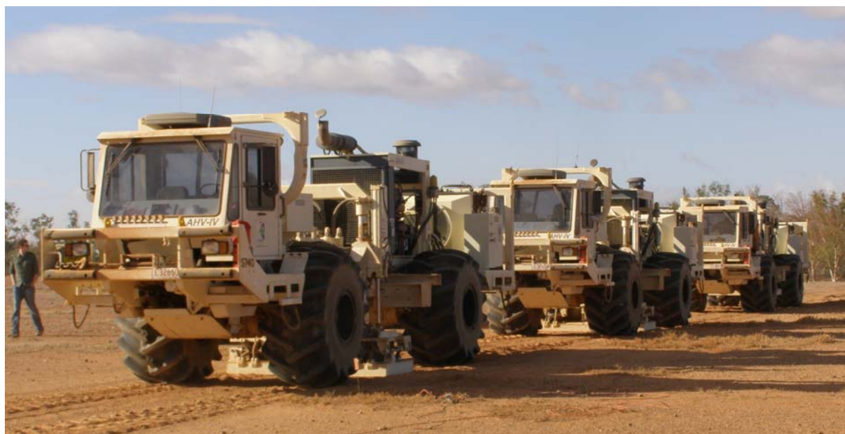
Figure 1. Vibroseis trucks in operation at Paralana
