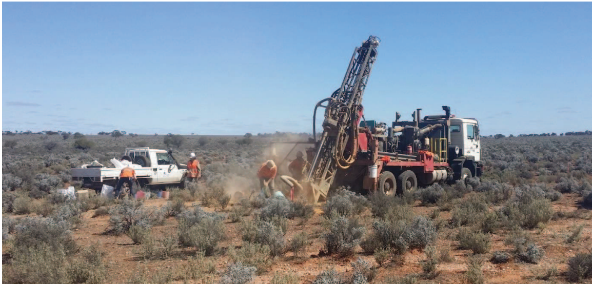
Figure 4 – Air core drill rig at Corunna.
