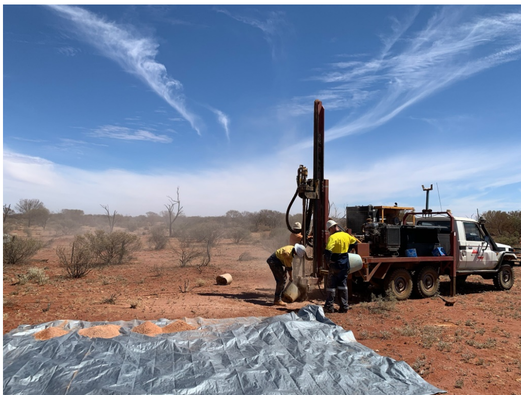
Photo: RAB Drilling Operations at Comet
