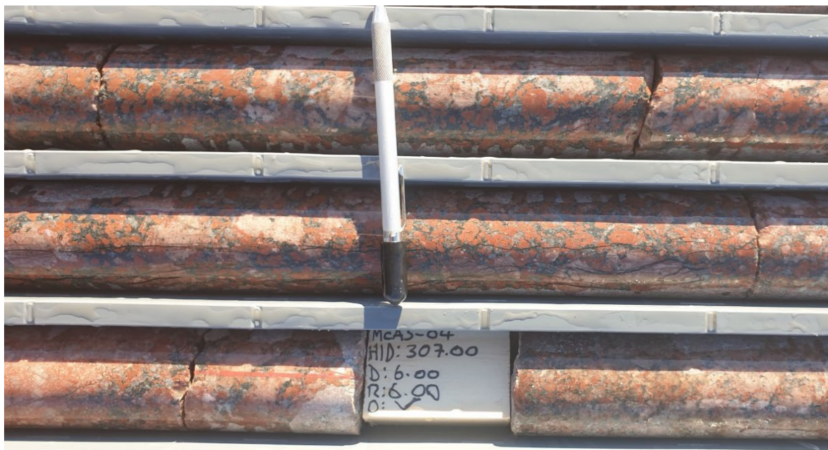
Figure 2 – Hole ID MCDA5-04 – Photo of core tray box 35, showing pervasive Red Rock (silica – hematized K-Feldspar (brick red)) alteration of original porphyritic granite host rock. Matrix of granite is enriched in the light rare earths, cerium, and lanthanum.
