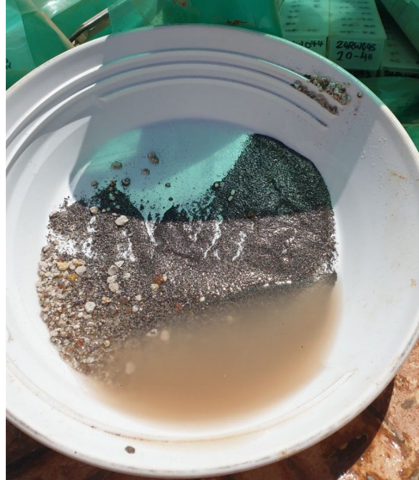
LEFT - High-grade Heavy Mineral Sand Interval - (drill hole 24RW049, 8-9m). Sands become distinctively dark grey due to high heavy mineral content. RIGHT – Panning of same interval highlights Heavy Minerals. HMC = 31.2%.
