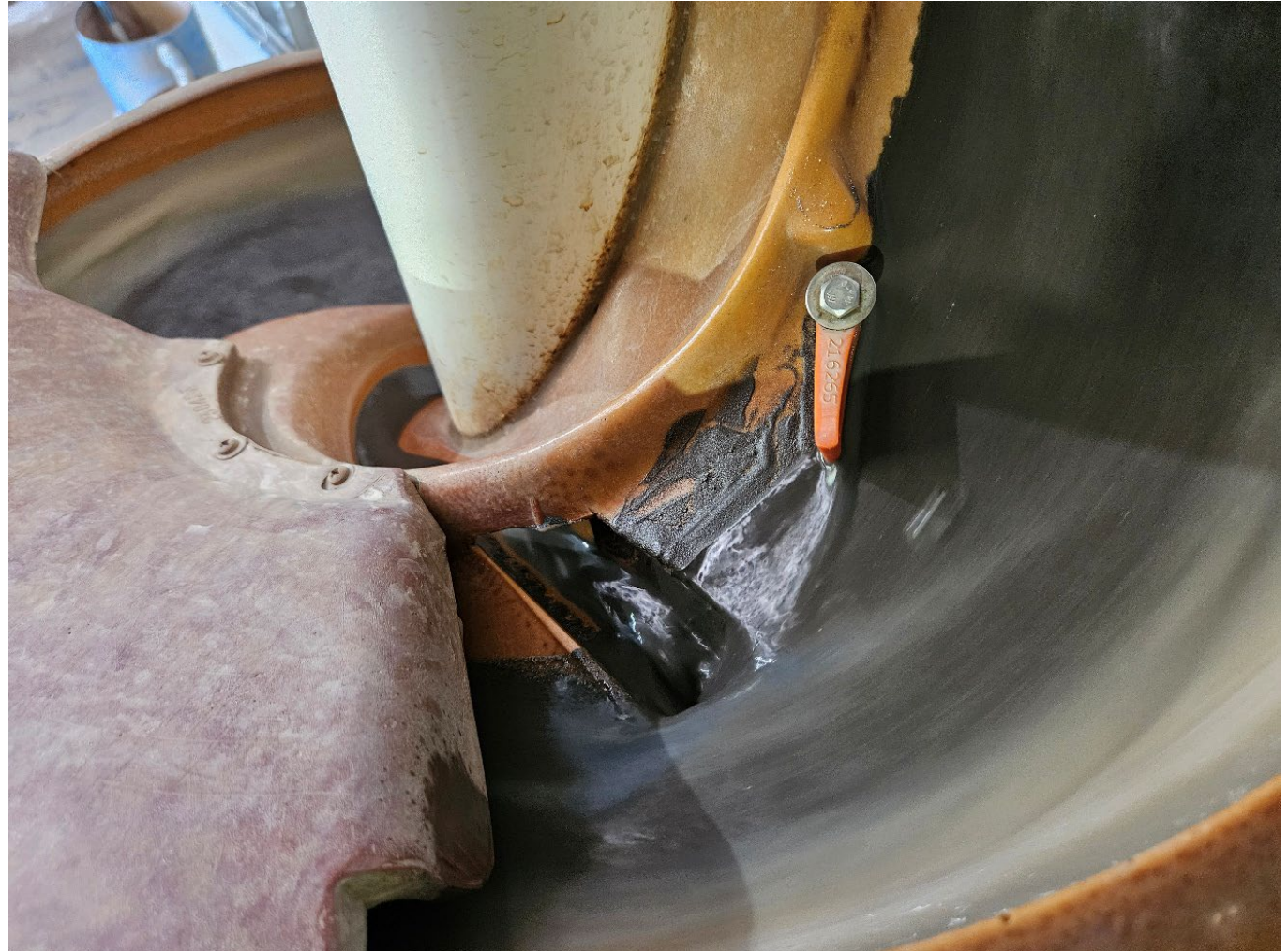
Rosewood HM sample being feed through a recleaner spiral at IHC Laboratories, Brisbane
