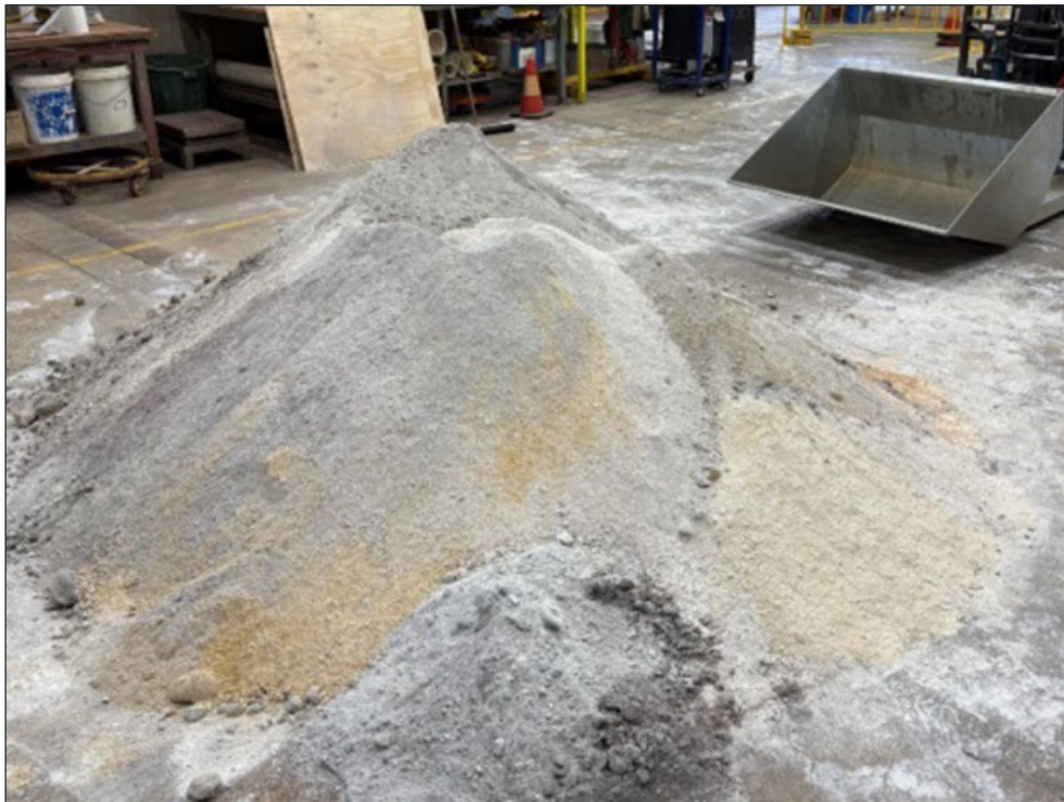
Figure 4: Three tonne bulk sample (RM04), averaging 13.0%HM, undergoing preparation for spiral separation
