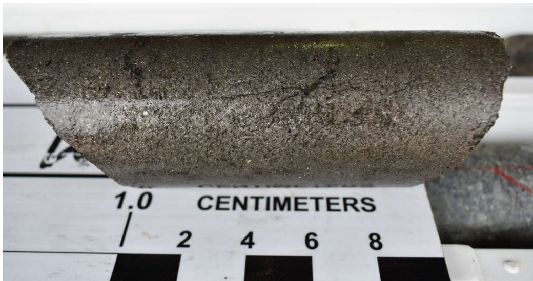
Figure 4: Massive sulphides 21WDD0004 130.5m downhole, pyrrhotite with smaller "shinier" pyrite and chalcocopyrite (greenish)
