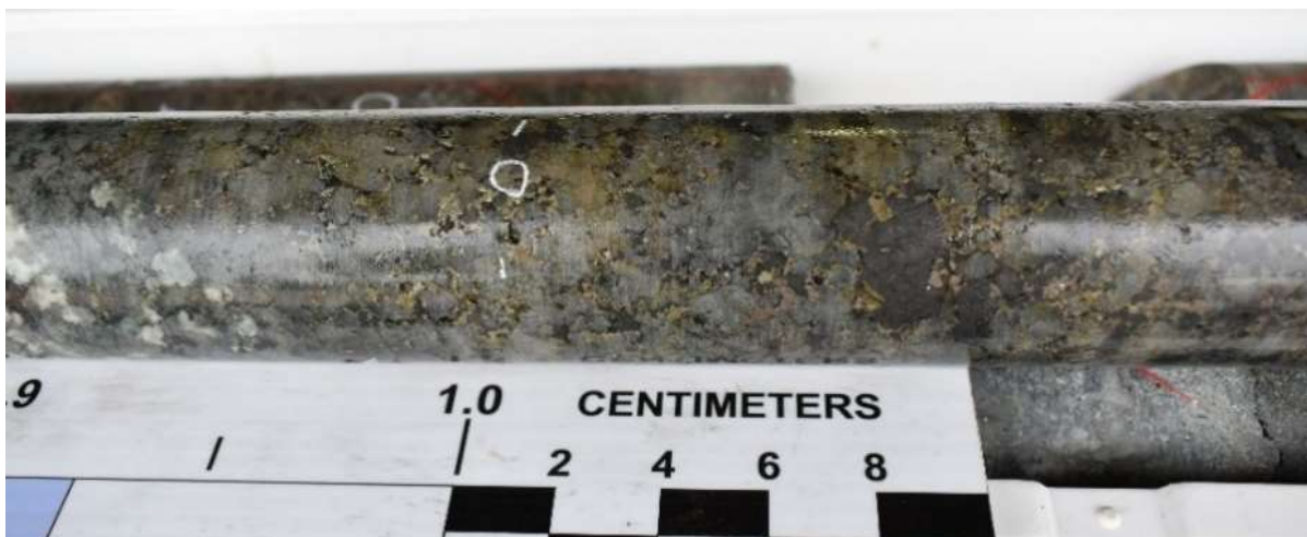
Figure 3: Felsic pegmatite intrusive 21WDD0004 - brecciation with pyrrhotite-pyrite-chalcopyrite-magnetite mineralisation as matrix at 123.7m
