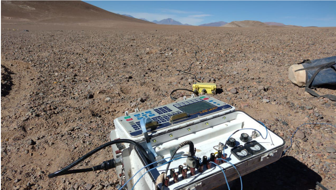
Figure 3 – CSAMT Station at the Rio Grande Sur Lithium Project
