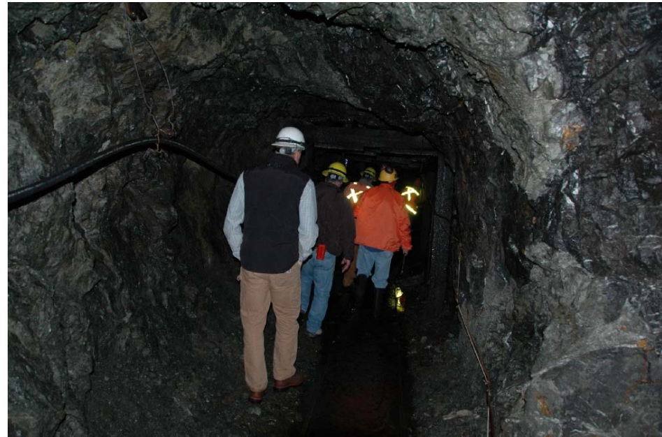
4630 level Adit at the Caribou Dome Copper Project. Grey material is an ash unit; black is mineralised sediment. Photo by Pierre Vella-Zarb.
