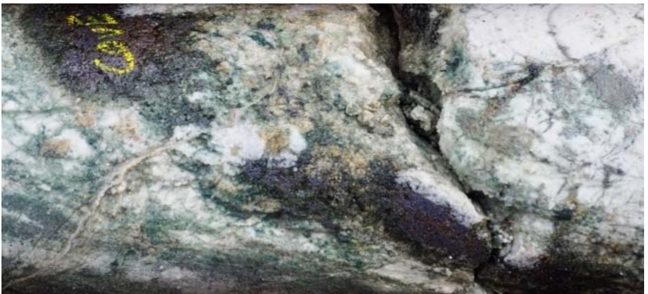
Figure 4 Covellite and Bornite bearing skarn, Hole ZM17008, 89.3m
