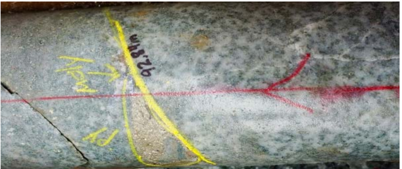
Figure 3 Early iron and molybdenum sulphides in dioritic endoskarn Hole ZM17010, 92.84m
