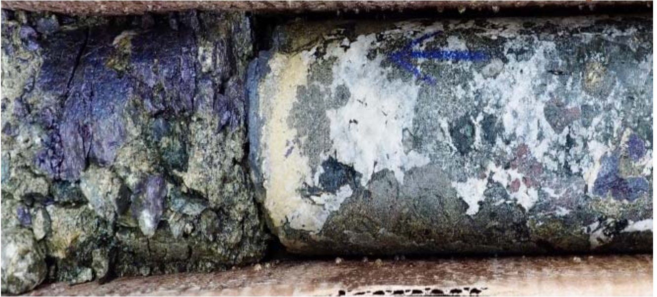
Figure 5 Bornite mineralisation in garnetiferous skarn, ZM17010, 179.4m
