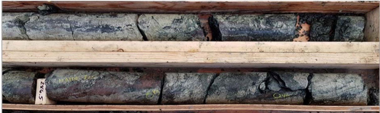
Figure 2. Visible magnetite, high-tenor copper sulphides and visible gold (circled) in hole ZX-18018 from 285.8m to 287.1m down-hole depth. Assay for this section was 3.2% Cu, 9.3 g/t Au and 38.2g.t Ag.
