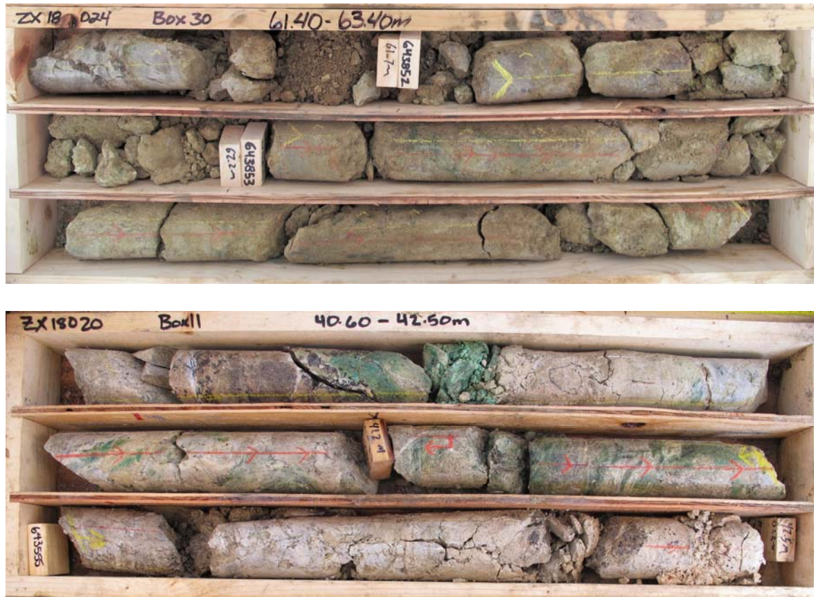
Figure 2. Visually similar styles of mineralisation in drill holes ZX-18024 (top) and ZX-18020 (bottom)
