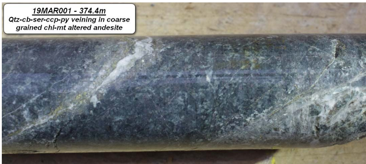
Figure 8 19MAR001 at 374.4m depth. Quartz-carbonate-sericite-chalcopryrite-pyrite veins in coarse grained chlorite-magnetite altered diorite.
