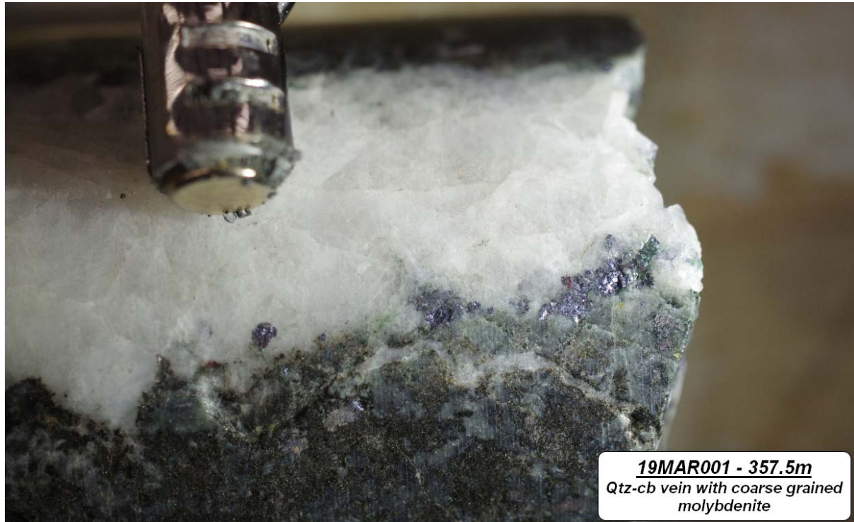
Figure 7 19MAR001 at 357.5m depth. Coarse-grained molybdenite in quartz-carbonate vein.
