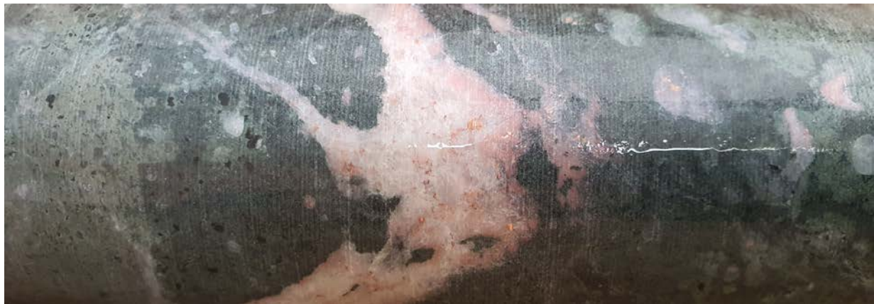
Figure 8 Coarse grained native copper blebs in rose quartz vein cutting porphyritic and vesiculated andesitic lava flow. 251.11m down-hole depth in drill hole CD21-007.
