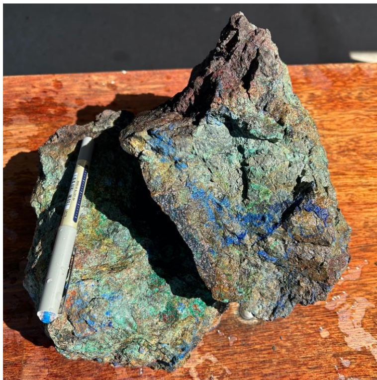
Figure 1: Oxidised gossan with supergene Cu (Azurite/Malachite) located at Mt Chalmers T1 prospect, pXRF scan 30.04% Cu .
