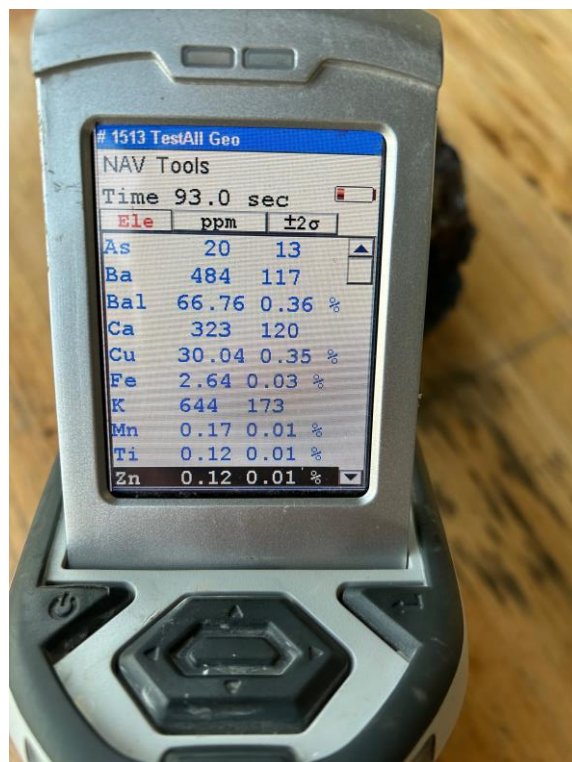
Figure 1: Oxidised gossan with supergene Cu (Azurite/Malachite) located at Mt Chalmers T1 prospect, pXRF scan 30.04% Cu .
