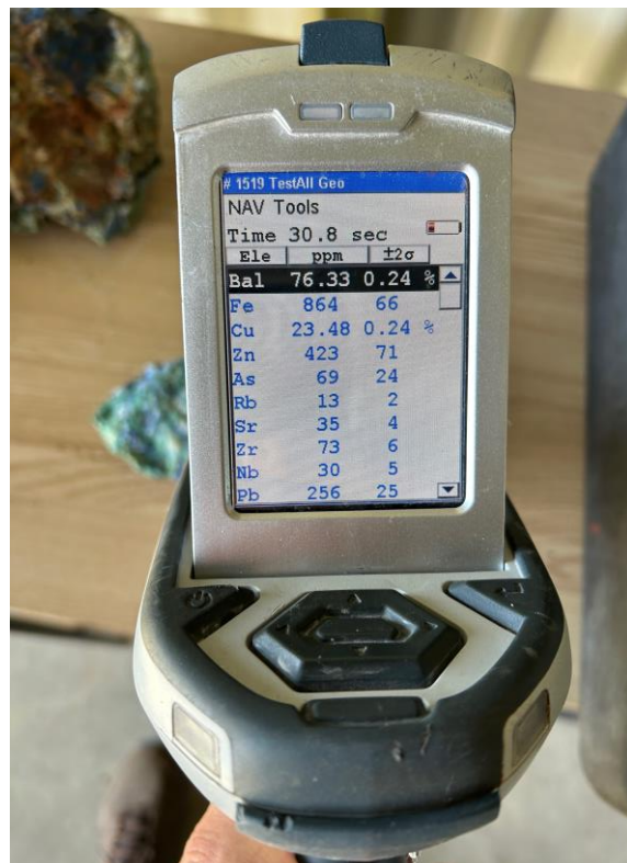
Figure 2: Quartz-carbonate breccia (Azurite/Malachite) located at Mt Chalmers T1 prospect, pXRF scan 23.48% Cu .
