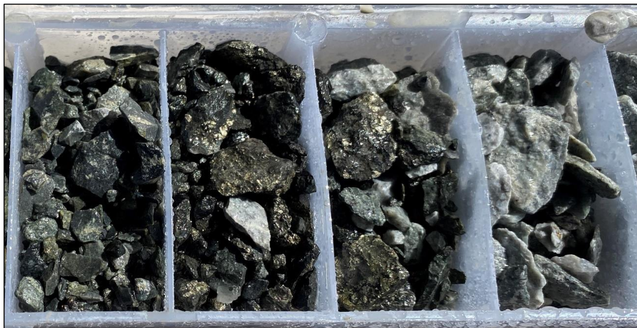
Figure 4: Cu-Zn Sulphides in RC chips, hole ARRC013, 230 – 234m.
