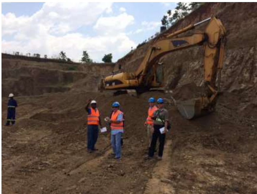
Photo 4: Open pit mining on ML4651 usea conventional owner operated standard truck and shovel operation
