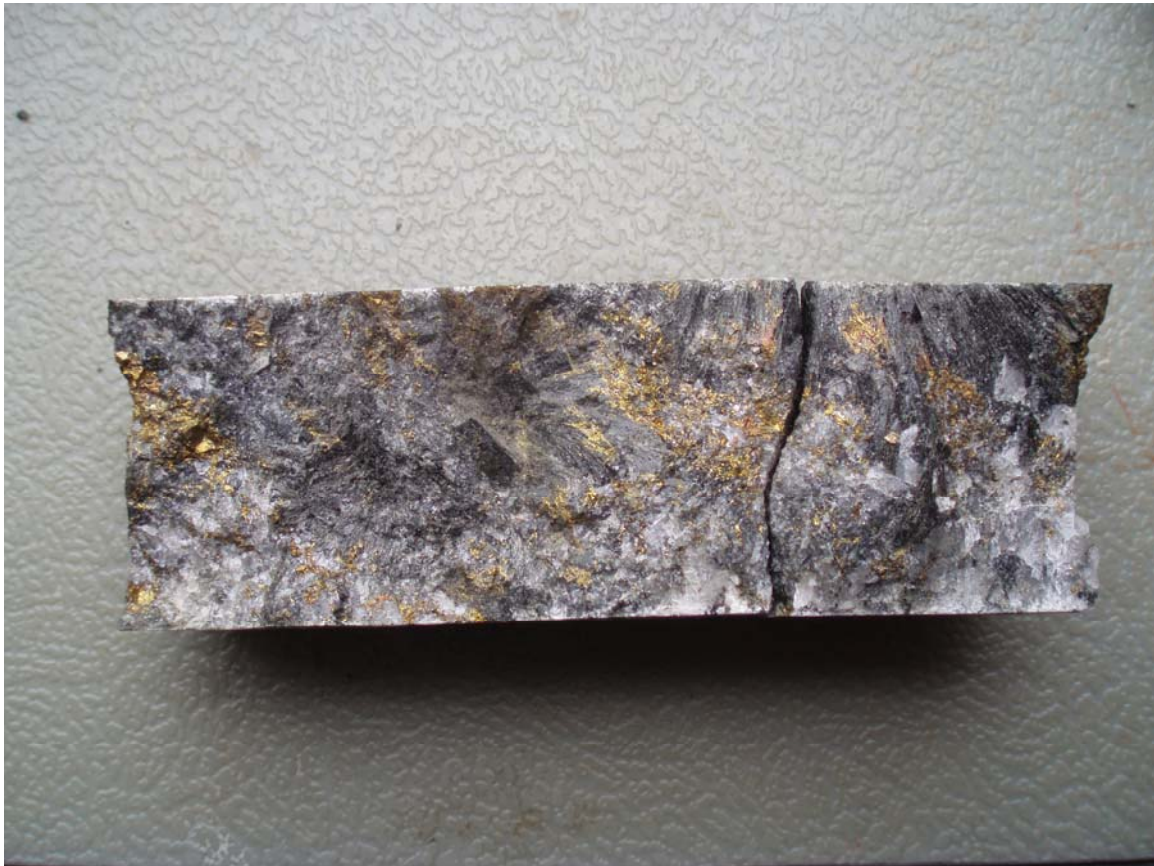
Past drill core from the Eastern Copper-Gold Zone, showing copper mineralisation
